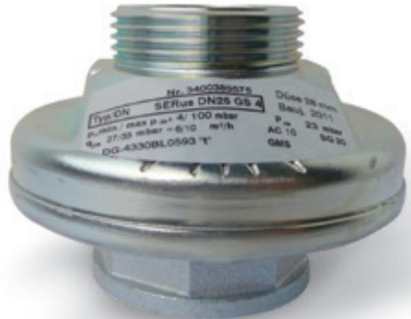
The SERus and SERus E residential regulators are based on a spring-loaded measuring unit. This type of regulator is used for direct pressure regulation at the inlet of residential and industrial gas meters.
