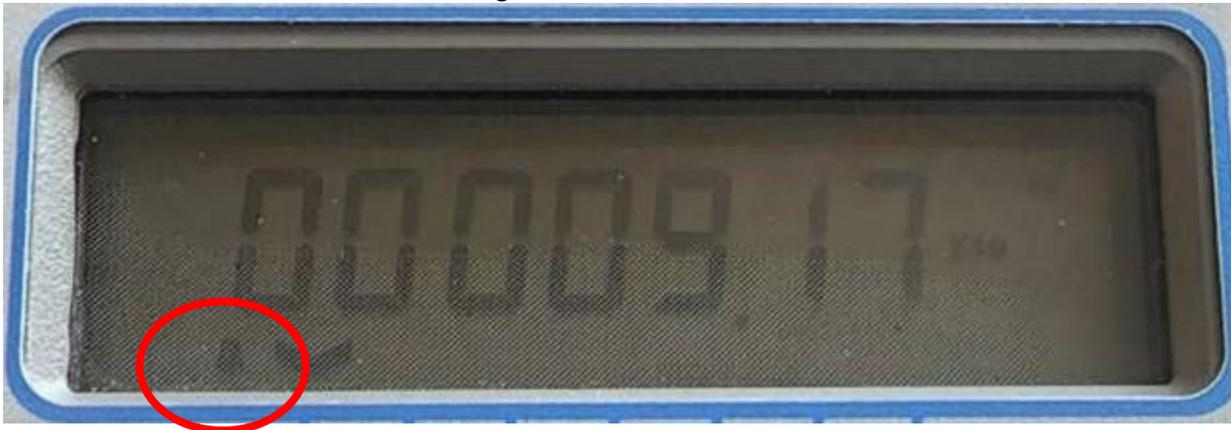
**Solid bell icon on display after a new digital transducer is connected to Micro Corrector**
