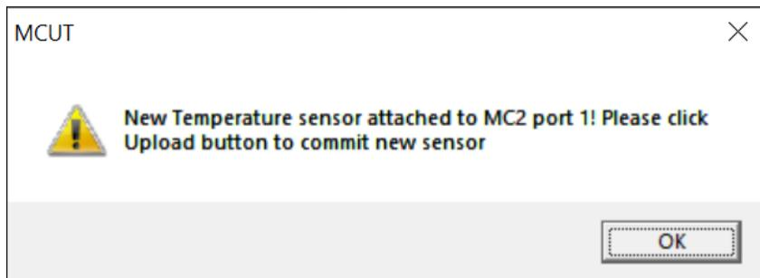
**Message in MCUT when a new temperature sensor is connected to the IMCW2 with either software password protection or metrological protection switch set in Read/Write position**
