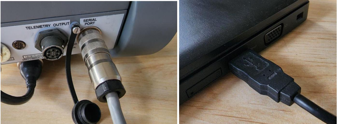
For direct communications connect the 9 way “D” type connector of the communications cable to COM port 1 on the PC; connect the round connector to the serial port connector located in the right-hand corner on the bottom of the IMCW2. If COM port 1 is not available, it is possible to specify which COM port is to be used within the MCUT for direct communication (**COM 1 to COM 255**). A fixed baud rate may be selected for modem communications.
