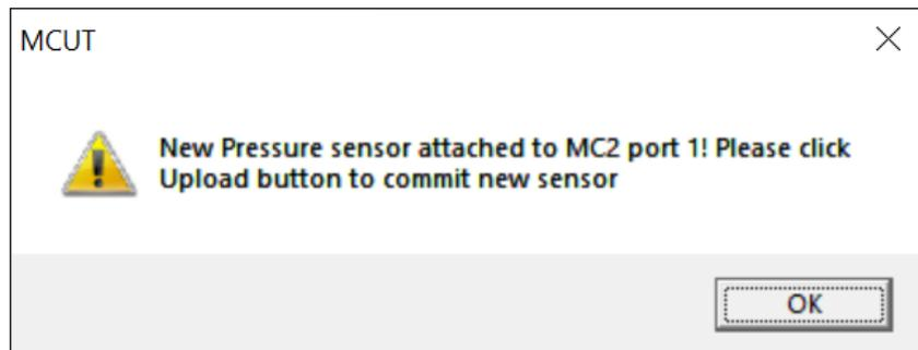
**Message in MCUT when a new pressure sensor is connected to the IMCW2 with either software password protection or metrological protection switch set in Read/Write position**
