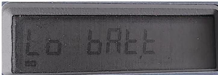
**Low Battery fault on display**
