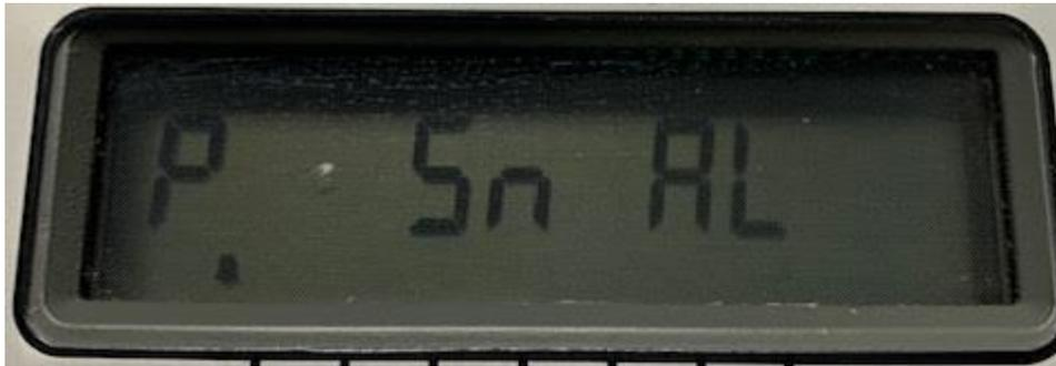
**Alarm indication on LCD when a new line pressure transducer is connected to the IMCW2**
