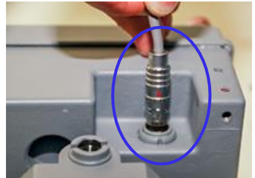
Figure 28: Push the AMR cable into the pulse output connector
