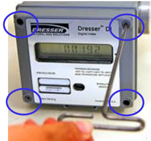
Figure 45: Remove four (4) screws on index cover
