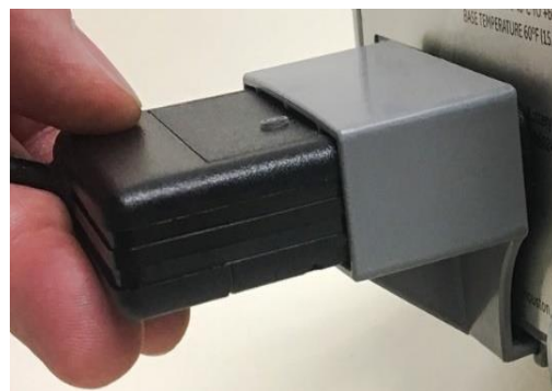
Figure 71: IR prover holder in slot
