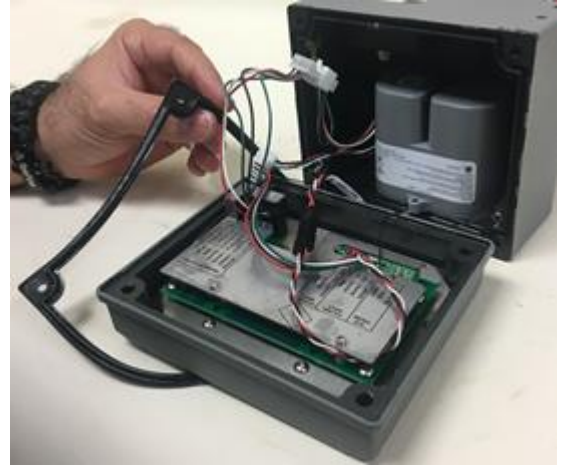
Figure 51: Remove the gasket
