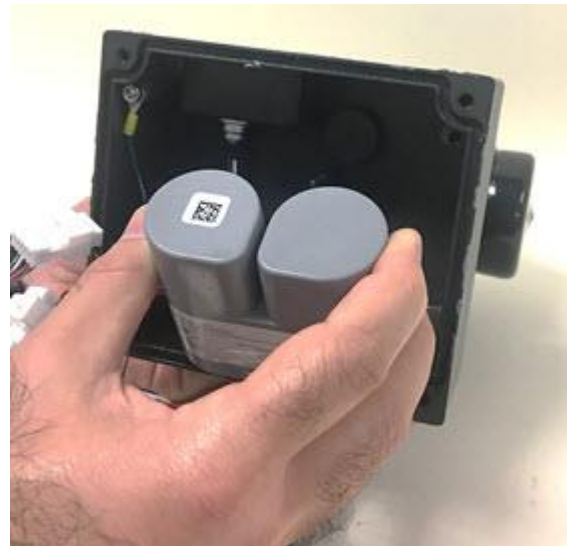
Figure 47: Pull the battery pack outwards
