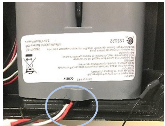
Figure 50: Insert battery pack with cable in channel
