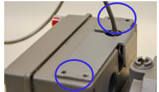
Figure 29: Align and attach the remote AMR mounting bracket to the digital index
