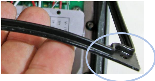
Figure 52: Closeup of gasket raised face side
