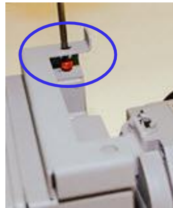
Figure 19: Align and attach the base AMR mounting bracket to the digital index
