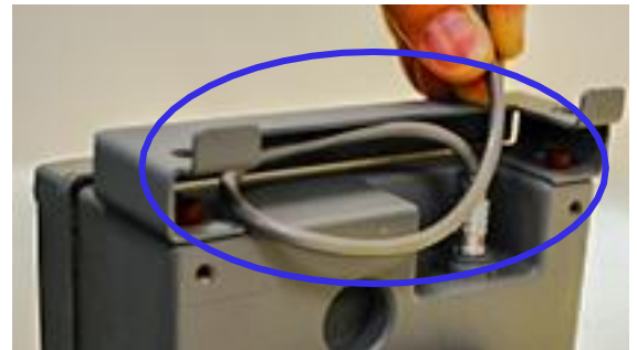
Figure 23: Tuck wires into base of AMR mounting bracket
