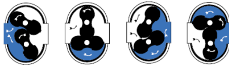
Figure 1: Two (2) contra-rotating impellers of two-lobe or ‘figure 8’ contour
