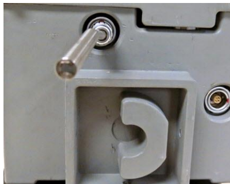
Figure 42: Temperature probe installation on digital index
