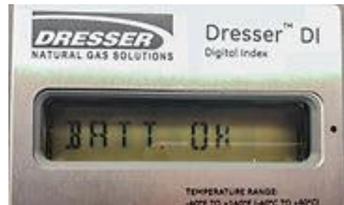
Figure 56: The battery is installed correctly
