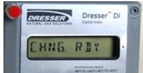
Figure 44: The battery is ready to be replaced
