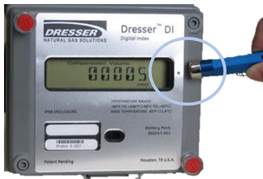
Figure 3: Magnet used to change screens
