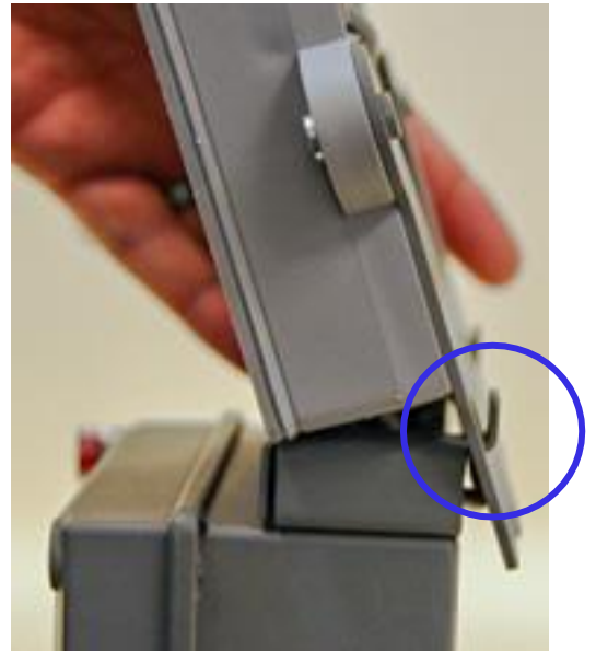
Figure 24: Slide on the top AMR mounting bracket
