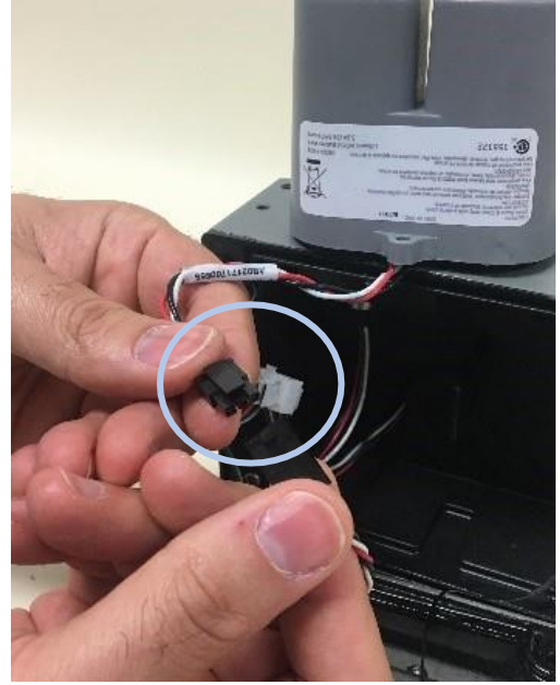
Figure 48: Disconnect/reconnect the wiring connector
