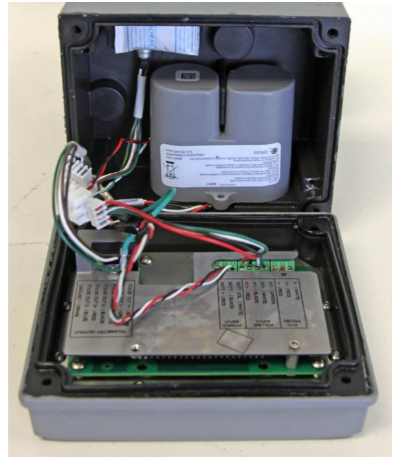
Figure 46: Remove the index cover
