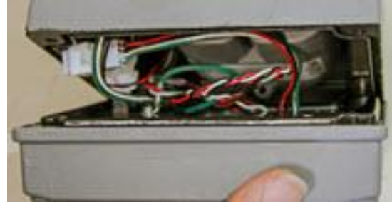
Figure 55: Tuck in all wires and replace the digital index cover (viewed from the top)
