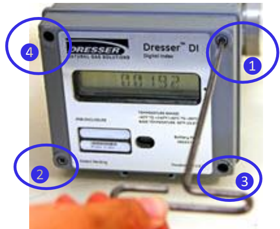
Figure 57: Insert and tighten cover screws
