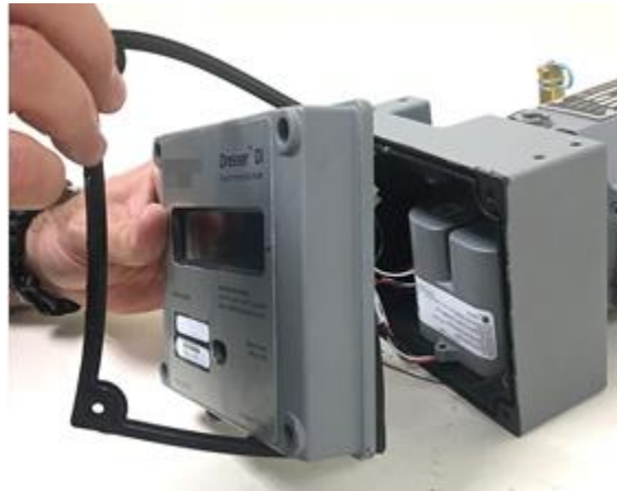
Figure 53: Replace the gasket
