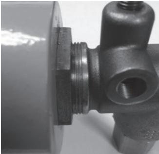
Three to five threads of the fluid head assembly should be visible once it has been installed onto the main pump body.
