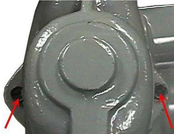
3. Carefully pull the diaphragm case away from the valve body. Inspect the valve seat, valve body and valve body gasket for any debris, damage, or deterioration. Replace the valve body gasket.
