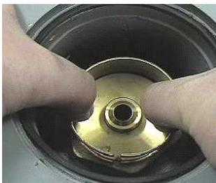
6. Remove the orifice using a 2 1/4-inch thin-wall socket wrench.
