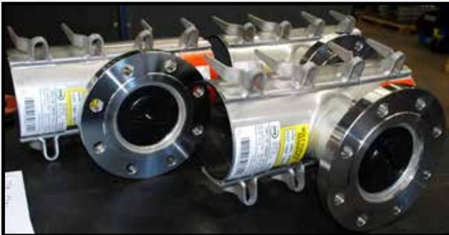
The Triple Tap Line Stop Fitting is available in sizes 4" thru 24" pipe diameters with both threaded or push plug design. And, like the Triple Tap Tapping Sleeve, it is designed to withstand the stresses and mechanical forces incurred during the line stopping process.
